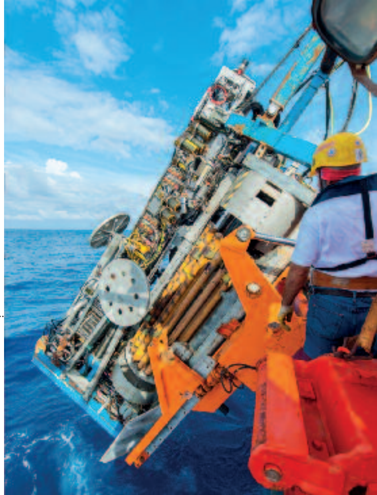
The MARUM-MeBo seafloor drill rig is launched from the SONNE research ship.
